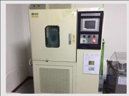
Multipath Temperature Tester (Junction Box For PV Module, Connector For Photovoltaic System)
