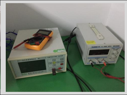
Multipath Temperature Tester (Junction Box For PV Module, Connector For Photovoltaic System)
